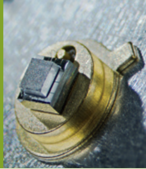
Figure 4: Flip-chip assembly on a silicon interposer, which is then attached to the TO submount
