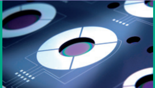
Drive electrodes for large aperture MEMS mirrors
