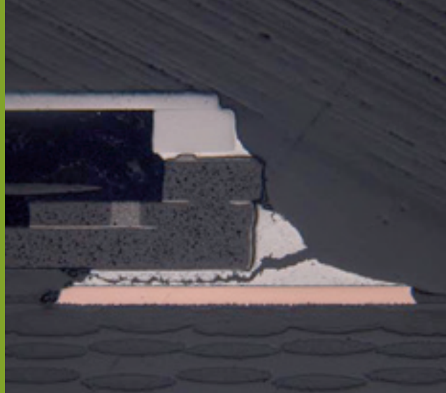
Figure 2: Component with crack in solder joint
