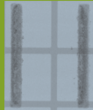
Figure 6: Crack growth BSA1 after 2000 temperature cycles
