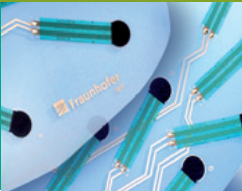
Foil sensors in functional shoe inlays for acoustic gait analysis
