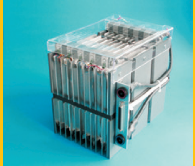
Figure 2: Single battery module used for construction of a 5 kWh storage system
